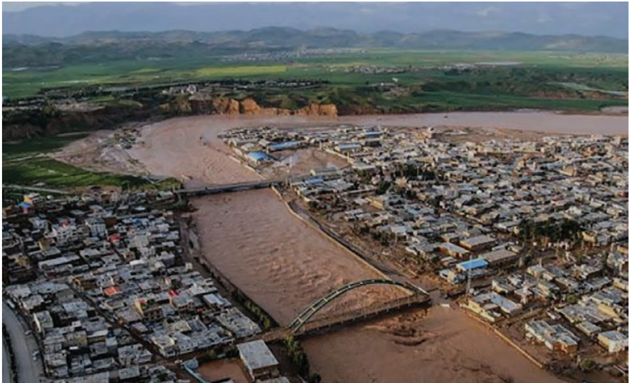
Image: Pol-e-Dokhtar in Lorestan Province was one of the cities that suffered the most damage in the 2019 floods. The newly built part of the city suffered the most damage due to the encroachment of the floodplain of the Kashkan River.
